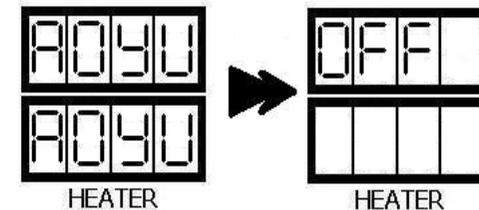
**NOTE:** *The product name may scroll more than once upon plugging the system to the power source. The system is trying to determine the appropriate operating frequency based on the user location. See Basic Troubleshooting Guide (page 14-15).*
